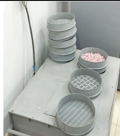
Figure 2. Methodology for optimizing the mesh surface of the seed cotton cleaner.
